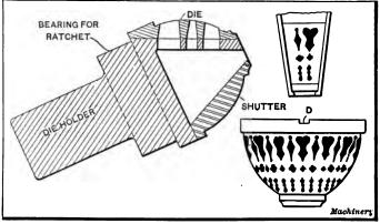
Fig. 11. Die and Holder for Perforating Shell shown to the Right
